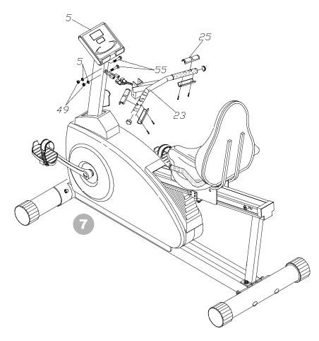
7. Attach the pulse wires in the front handlebar (23) to the wires from the console (5). Connect the front handlebar (23) to the console tube with the locknuts (49), flat washers (50) and screws (55) provided. Make sure not to "pinch" any of the pulse wires when connecting the handlebar to the console tube.
